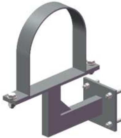
Support and clamp when firewall exists Figure 114: Oil Drain Pipe Support Example
