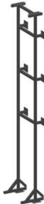
Support to be attached to the transformer firewall Figure 120: EGOST Support
