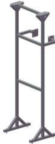
Support to be attached to the transformer
