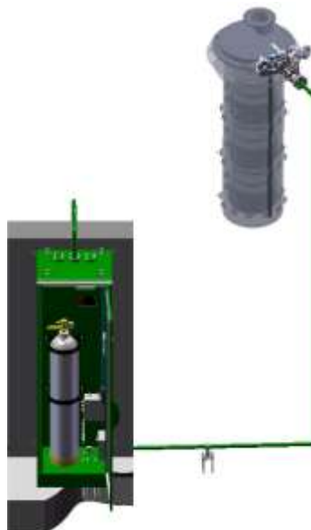
Figure 110: Inert Gas Injection Pipe routed from the TP Cabinet to the OLTC
